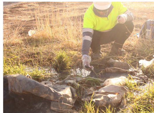
Monitoring pH prior to construction using a handheld instrument in the field.
